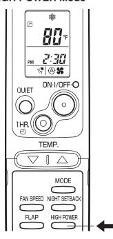
HIGH POWER mode can be used to increase the output of the indoor unit for all operation modes.
